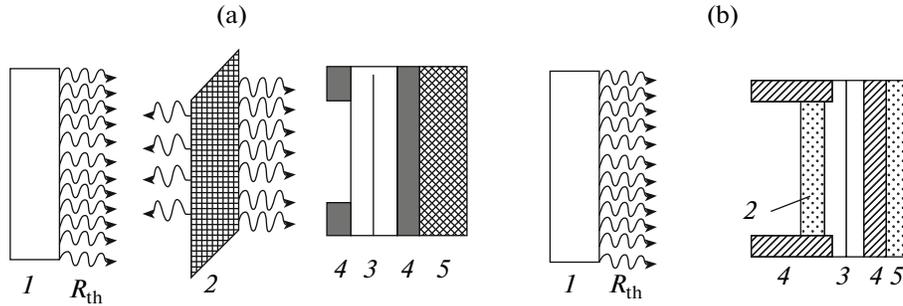
**Fig. 1.** (a) Main parts of a thermophotovoltaic facility: (1) thermal radiation source; (2) selective emitter (or reflector – filter); (3) photoelectric cell,  $p$ – $n$  junction; (4) ohmic contacts; (5) radiator; (6) thermal radiation,  $R_{th}$ . (b) Parts of a photothermoemovoltic facility: (1) thermal radiation source; (2) photothermoelectric cell–transparent heat insulation layer; (3)  $p$ – $n$  junction; (4) ohmic contacts; (5) heat insulation layer.
