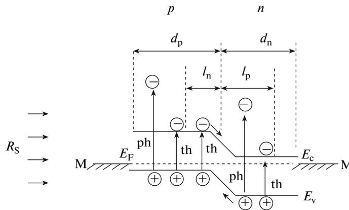
**Fig. 2.** Schematic diagram illustrating the band structure at the  $p$ – $n$  junction of a photothermoelectric cell: M are metallic contacts; ph and th are photo- and thermoexcitation of eh pairs, respectively;  $l_n$  and  $l_p$  are diffusion paths of electrons and holes, respectively;  $d_n$  and  $d_p$  are widths of the  $n$  and  $p$  layers, respectively;  $R_S$  is solar radiation.
