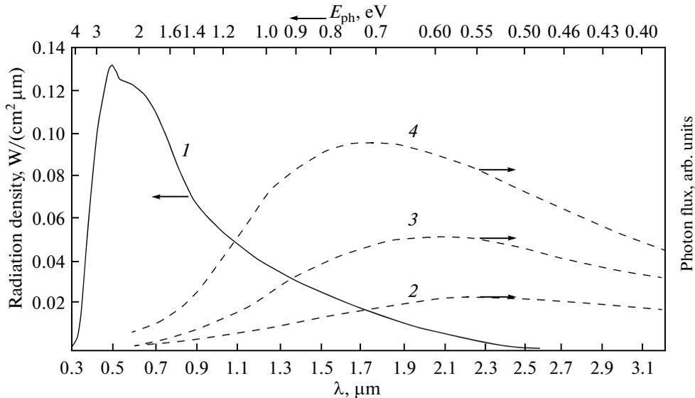
**Fig. 3.** (1) Spectral distribution of the solar radiation at the sea level in the case of clear sky; (2–4) photon flux densities for black-body radiation corresponding to 1300, 1500, and 1700 K, respectively.
